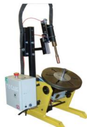
High production automatic MIG welding of small circular parts for automotive industry.
